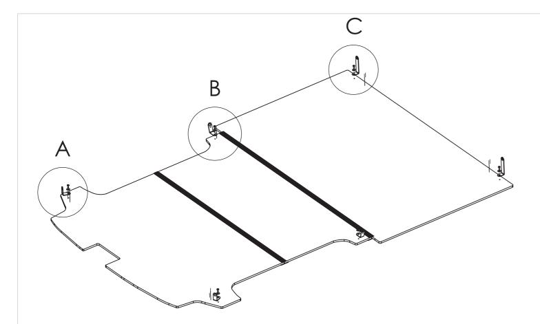
STEP 4 : FIT BRACKETS PTKTFFTCSWBB01, PTKTFFTCSWBB02 AND PTKTFFTCSWBB03 INTO POSITIONS AS SHOWN USING THE EXISTING CARGO TIE DOWN POINTS.
