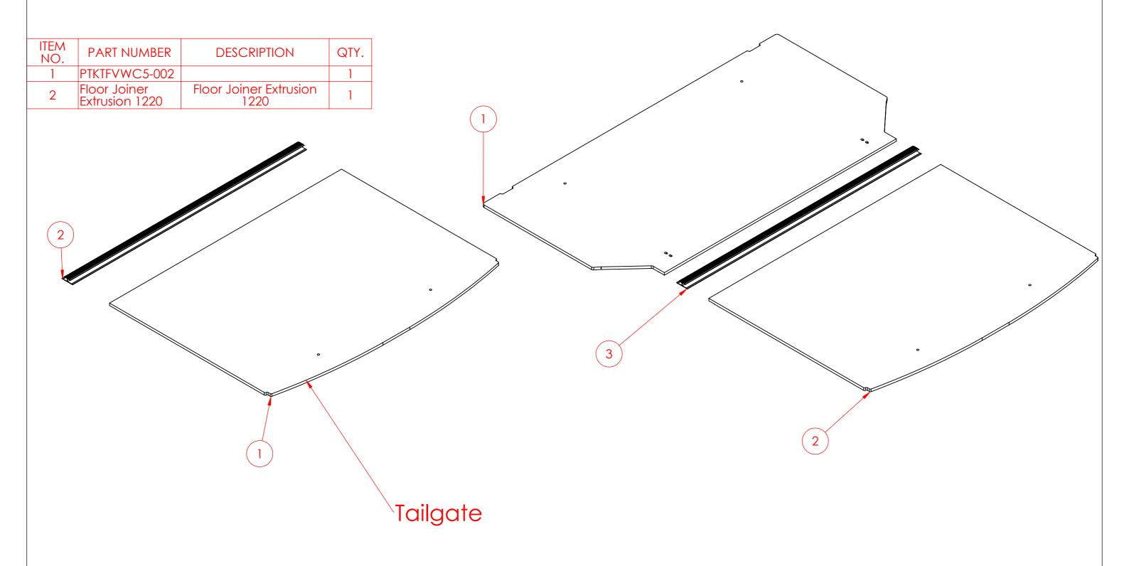
UNLESS NOTED OTHERWISE DIMENSIONS IN MILLIMETRES Project: PTKT Floor DRAWING APPROVAL Snr.Management: Client: Revision: DO NOT SCALE Status: Approved Material: Thickness: Date: 31/10/2024 Print Date: Part No:PTKTFVWCAD21-KIT aut safe PROPRIETARY AND CONFIDENTIAL Vehicle: VW Caddy 21 Scale: SCALE:1:20 Sheet Size: A3 Finish:Refer Production file THE INFORMATION CONTAINED WITHIN THIS
