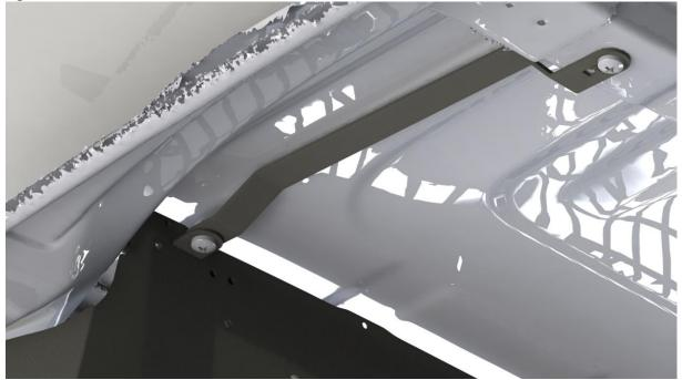
6. Separate spacer from tie point bracket assembly and insert spacer into original hole in b post rim panel. Attach SPLDVED7-007 to partition using M10x30 Set Screw and M10 Whiz nut. Do not fully tighten. Attach bracket back to vehicle body using original tie point bolt.
