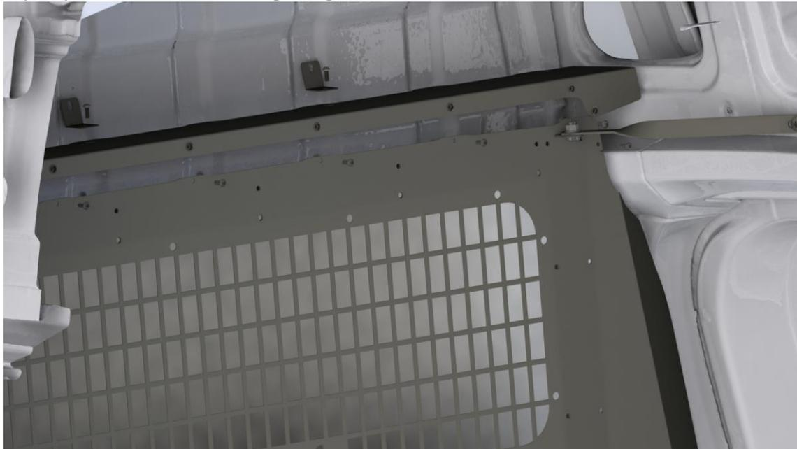
8. Centralize partition and fully tighten all bolts.
