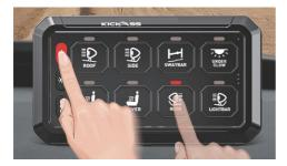
Use the switch panel to operate the loads. Press the red button to power on the switch panel, then use the switch buttons to turn devices on or off.
