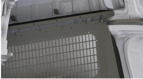
8. Centralize partition and fully tighten all bolts.
