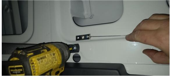
6. Separate spacer from tie point bracket assembly and insert spacer into original hole in b post trim panel. Attach SPLDVED7-007 to partition using M10x25 Set Screw and M10 Whiz nuts. Do not fully tighten. Attach bracket back to vehicle body using original tie point bolt.
